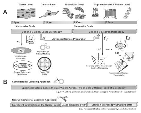
Fig. 1. Scheme illustrating the concept of correlative multidimensional light (3-D) or confocal laser optical imaging (4-D) with electron microscopy (2-D or 3-D) imaging (Reprinted with permission from, [5]). A: Depending on the sample source (e.g., tissue
